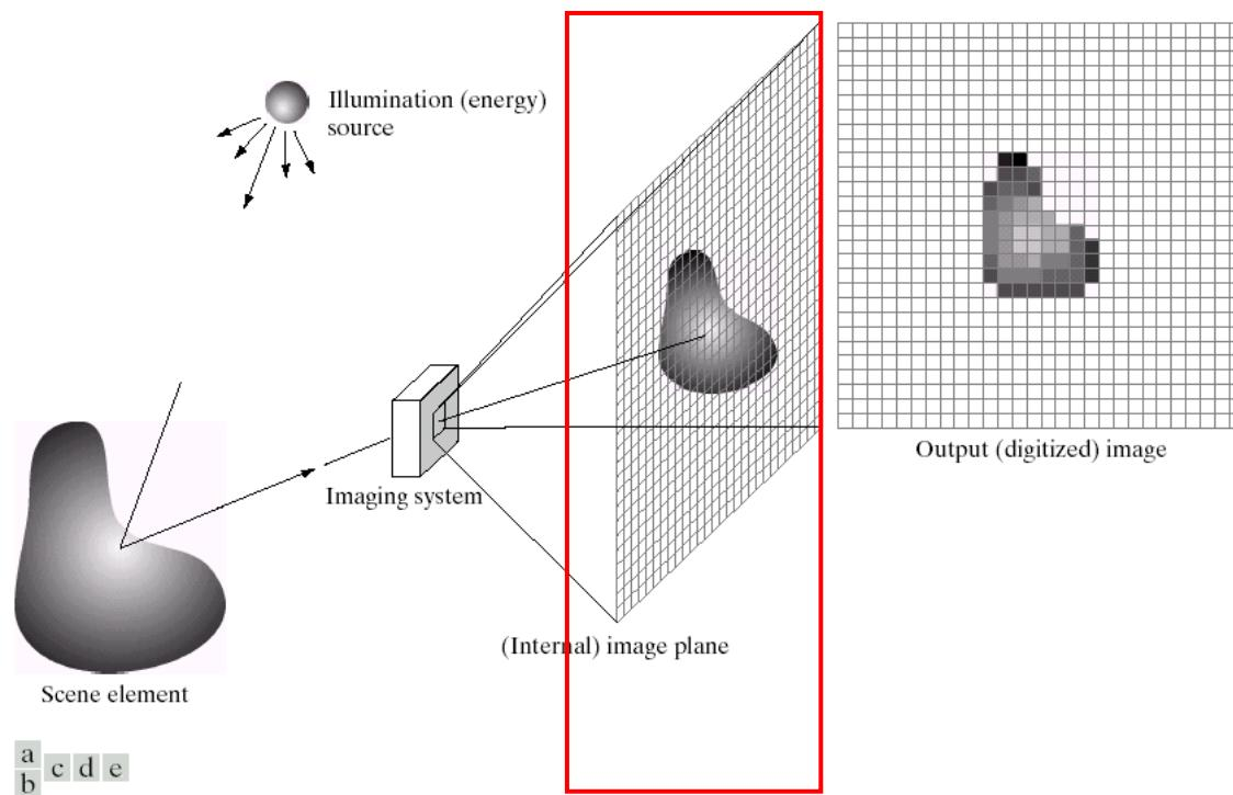
**FIGURE 2.15** An example of the digital image acquisition process. (a) Energy (“illumination”) source. (b) An element of a scene. (c) Imaging system. (d) Projection of the scene onto the image plane. (e) Digitized image.
